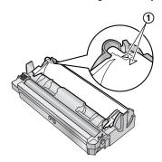
**11** Install the drum and toner unit (①) by holding the tabs.
